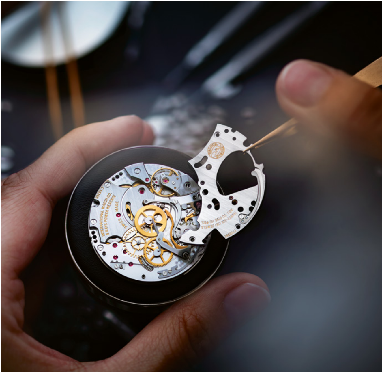
The watch bridge is mounted onto the movement
