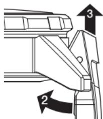
Tilt the bracelet or strap inwards (2) and move it upwards away from the case (3).
