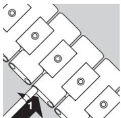
Repeat steps 1 to 3 at the distance from the first point of separation you have just determined. Remove the unnecessary links and reassemble the shortened bracelet. Slide the hinged link into the bracelet sideways (1).
