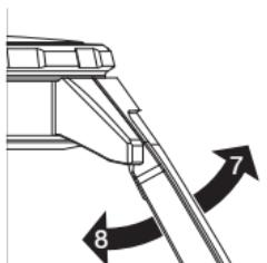
After changing the strap, please ensure that it is securely attached by pulling both sides up (7) and down (8) firmly.
