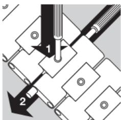
Open the folding clasp by pressing the buttons on the side. Lay the bracelet face down on a firm base. To avoid scratching the bracelet and base, place a cloth underneath the bracelet. Using the special tool provided, you can now push down the fixing bolt at the desired point of separation (1) and at the same time, slide the hinged link with the help of the second tool about 3 millimetres sideways (2).
