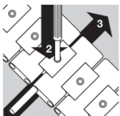
Using the special tool provided, you can now push down the fixing bolt (2) and at the same time, slide the hinged link back into the bracelet until it lies flush (3).
