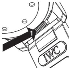
Your Aquatimer Automatic comes with a patented IWC bracelet quick-change system that enables you to change the bracelet or strap quickly and simply, without the use of tools. To remove the bracelet or strap, use your thumbnail to firmly push the retaining lever (1) located on the underside of the horns outwards.
