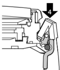
To attach the bracelet or strap, hook the notch of the horns from above into the spring pin of the case (4).
