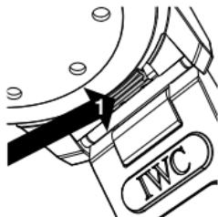
Your Aquatimer Automatic 2000 comes with a patented IWC bracelet quick-change system that enables you to change the bracelet or strap quickly and simply, without the use of tools. To remove the bracelet or strap, use your thumbnail to firmly push the retaining lever (1) located on the underside of the horns outwards.
