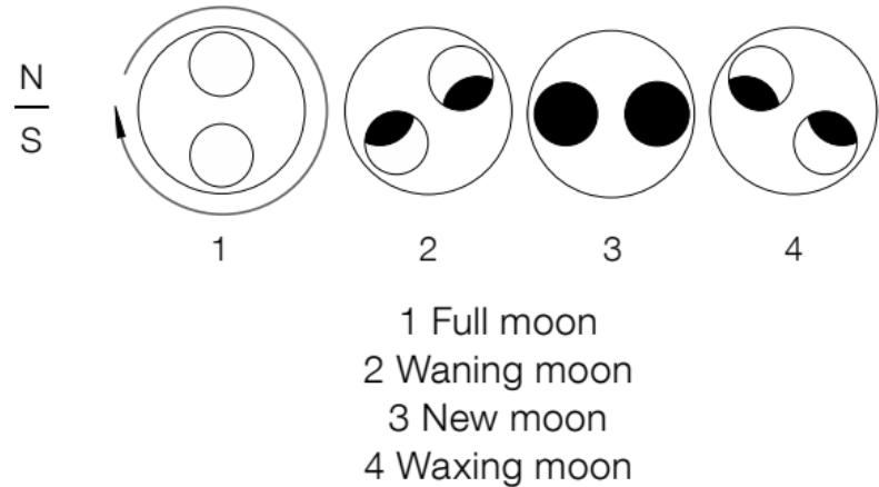
The moon phase display is automatically set by the calendar so that it is always correct. The transmission ratio is so
