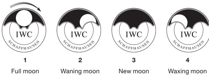
The moon phase display is automatically set by the calendar so that it is always correct. The transmission ratio is so precise that the display deviates by only a single day after 577 years.
