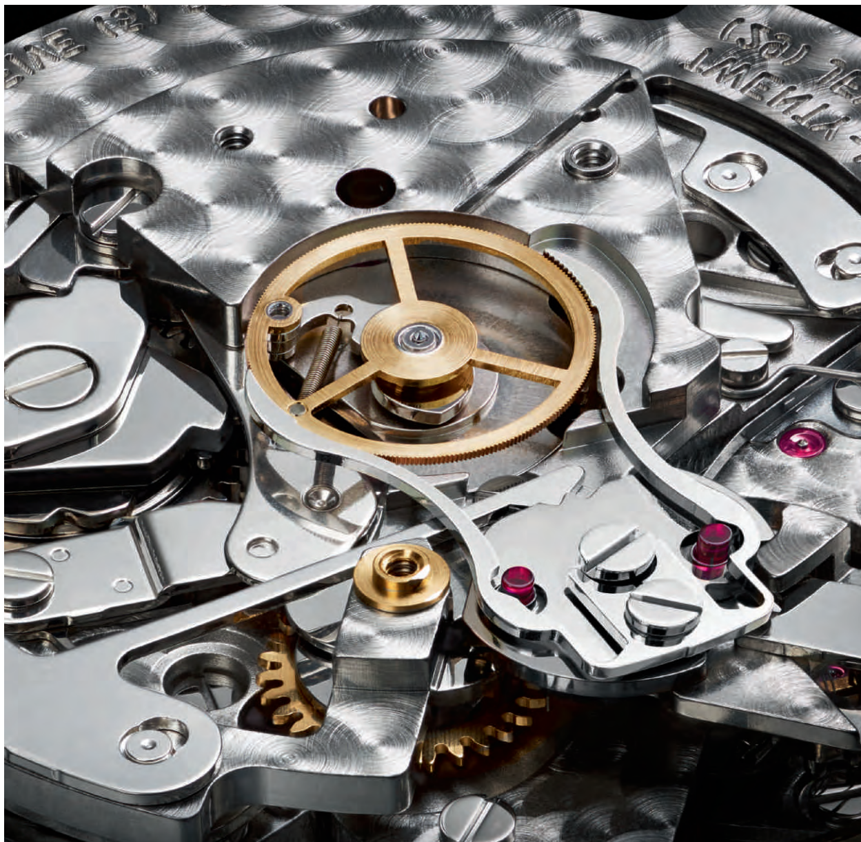
In a rattrapante mechanism, the split-seconds hand starts simultaneously with the stopwatch hand
