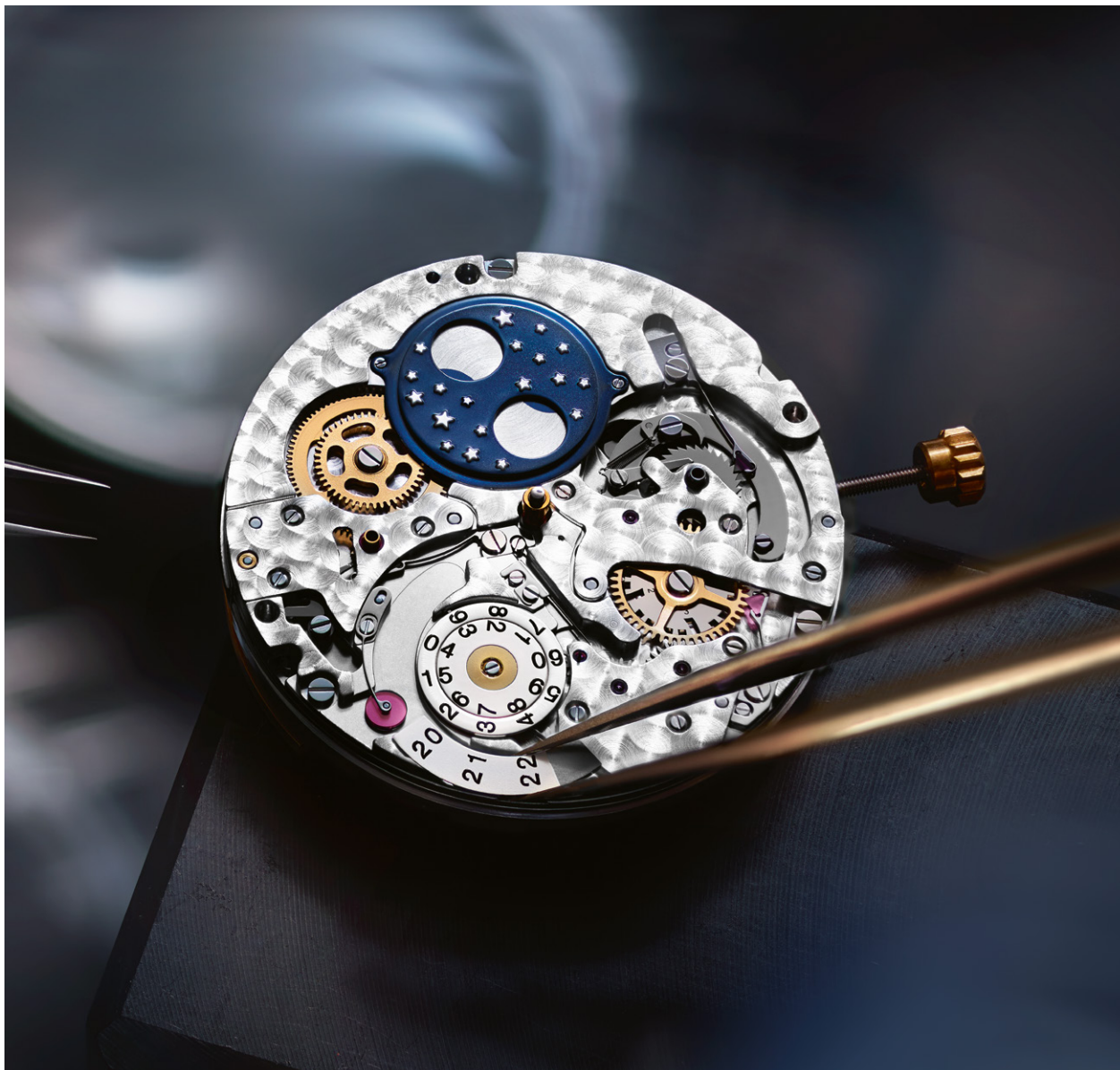
The IWC perpetual calendar also takes the leap years into account: the century slide supplied with the watch will go on showing the year correctly until 31 December 2499
