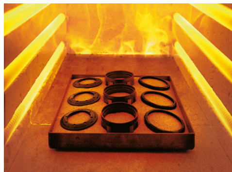
During the sintering process, the surface of Ceratanium® not only takes on the features typical of ceramic but also receives its unique matte black colour
