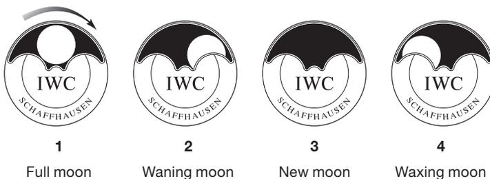
The moon phase display is automatically set by the calendar so that it is always correct. The transmission ratio is so precise that the display deviates by only a single day after 577 years.
