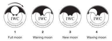
The moon phase display is set automatically by the date-mechanism and is thus always correct. The reduction ratio is so precise that the display will only deviate by a single day after 577 years.
